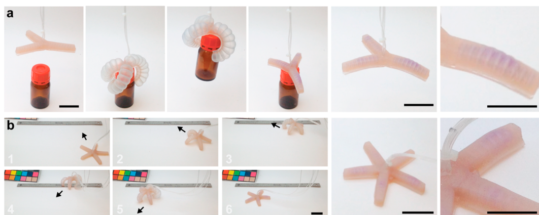
Figure 3. Three-arm gripping robot (a) and five-arm walking robot (b) are shown. Initial robots (left) are inflated to produce a color change when network stresses/strains reach a critical value. The color persists for several minutes after the robot is returned to the initial state (right). The inset numbers indicate the temporal order of the images. Scale bars = 5 cm.
